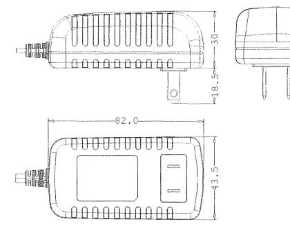
NOTE:1. Case cover & chassis material: PC/ABS (UL94V-1) BLACK
