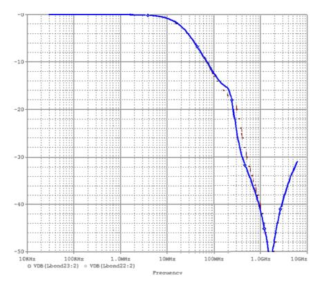
Figure 4. Attenuation Curve for CM1454 RC Filters: 3, 4, and 5
