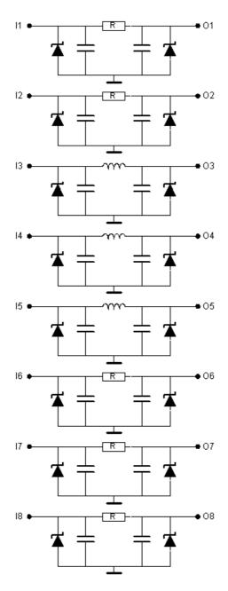
Figure 1. CM1454 Schematic Diagram of R-C and L-C Filter Arrays with ESD
