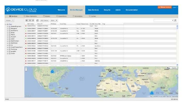
From the Device Manager interface, you can configure devices, remotely update device firmware, upload and manage Python/DIA files, remotely reboot devices, reset devices to factory defaults, backup/restore device configuration properties, import or export the device configuration properties, track devices, monitor devices and connections.
