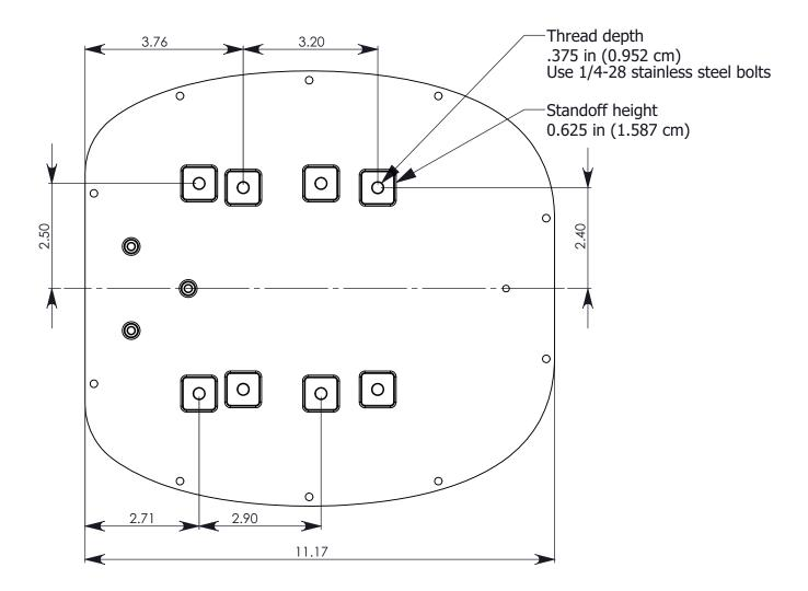
Use eight 1/4-28 stainless steel bolts to mount the ConnectPort X5 Fleet unit. Use a bolt length such that the bolt does not penetrate into the ConnectPort X5 Fleet unit by more than a thread depth of .375 in (0.952 cm).
