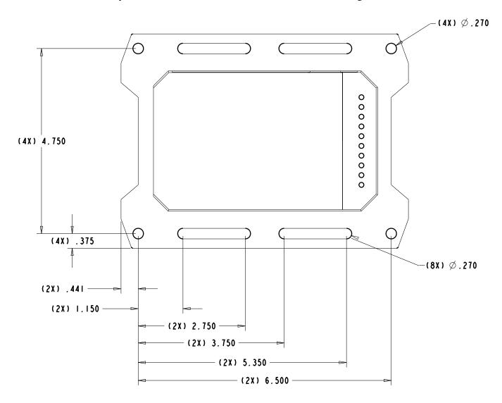
Use at least four (4) ¼" bolts to mount the ConnectPort X5 R unit. The ConnectPort X5 R unit is IP67 rated; allowing for it to be mounted inside or outside. The ConnectPort X5 R enclosure is made of CEP-coated aluminum, and the TNC connectors and nuts are made of nickel-plated brass.
