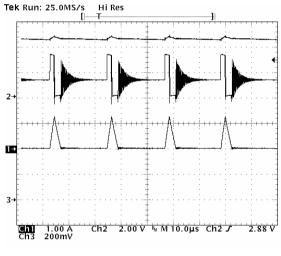
Ch1-> Inductor current Ch2-> Phase Node Ch3-> Output voltage
