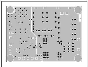
Figure 21. Power & signal plane
