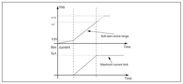
Figure 8. Soft -Start Diagram
