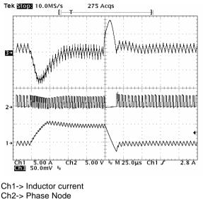
Ch2-> Phase Node Ch3-> Output voltage
