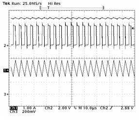
Ch1-> Inductor current Ch2-> Phase Node Ch3-> Output voltage
