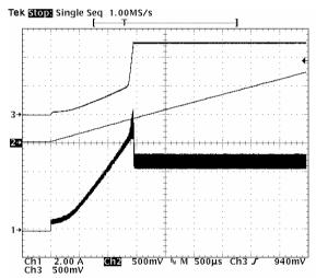
Ch1-> Inductor current Ch2-> Soft start Voltage Ch3-> Output voltage
