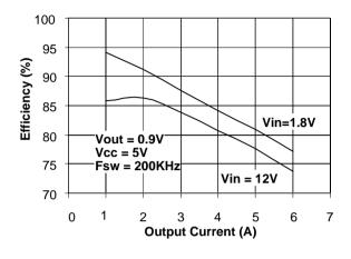
Figure 28. Eff. vs. Output Current Source Mode
