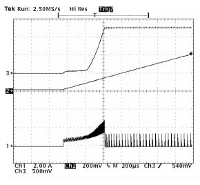
Ch1-> Inductor current Ch2-> Soft start Voltage Ch3-> Output voltage
