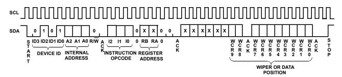
FIGURE 7. FOUR-BYTE INSTRUCTION SEQUENCE (WRITE OR READ FOR WCR OR DATA REGISTERS)
