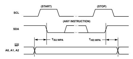
FIGURE 12. WRITE PROTECT AND DEVICE ADDRESS PINS TIMING
