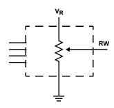
FIGURE 13. THREE-TERMINAL POTENTIOMETER; VARIABLE VOLTAGE DIVIDER
