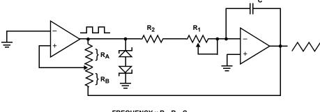
FREQUENCY  $\mu$   $R_1,\,R_2,\,C$  AMPLITUDE  $\mu$   $R_A,\,R_B$
