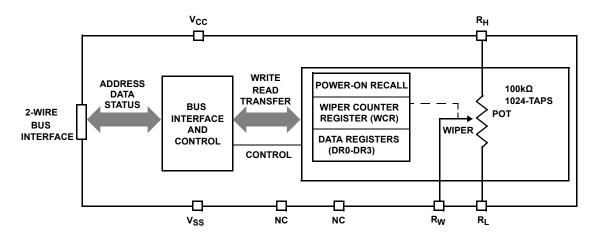
FIGURE 1. FUNCTIONAL DIAGRAM
