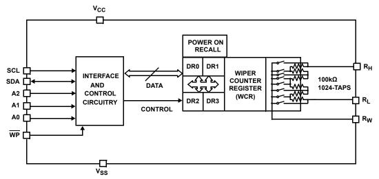
FIGURE 2. DETAILED FUNCTIONAL DIAGRAM
