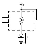
FIGURE 14. TWO-TERMINAL VARIABLE RESISTOR; VARIABLE CURRENT
