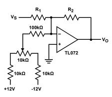
FIGURE 17. OFFSET VOLTAGE ADJUSTMENT
