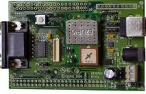
The EZURiO Development Kit is designed to support the rapid development of hardware, applications and software for the EZURiO range of BISM II Bluetooth Intelligent Serial Modules and WISM Wireless LAN modules. The EZURiO development kit is available in five options to cover the widest range of wireless technologies, including hardware support for development of applications for the Siemens MC55 GSM GPRS modules.
