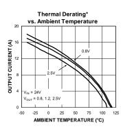
**Die Temperature\***: The temperature measurement was taken at the hottest point on the MIC26950 case mounted on a 5 square inch 4 layer, 0.62", FR-4 PCB with 2oz finish copper weight per layer, see Thermal Measurement section. Actual results will depend upon the size of the PCB, ambient temperature and proximity to other heat emitting components.
