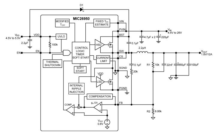
Figure 1. MIC26950 Block Diagram
