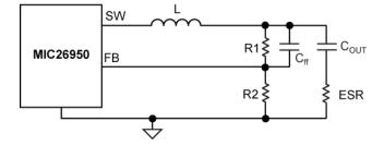
Figure 5b. Inadequate Ripple at FB
