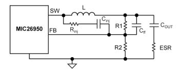
Figure 5c. Invisible Ripple at FB
