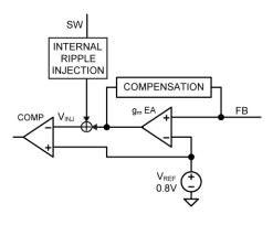
Figure 7. Internal Ripple Injection
