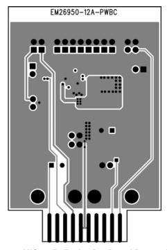
Figure 12. MIC26950 Evaluation Board Bottom Layer
