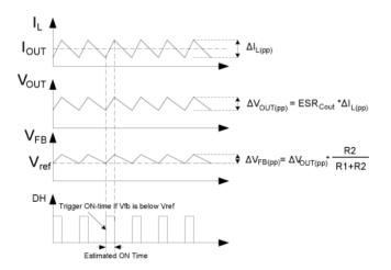
Figure 2. MIC26950 Control Loop Timing
