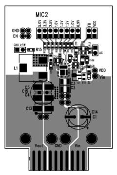
Figure 9. MIC26950 Evaluation Board Top Layer
