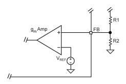
Figure 6. Voltage-Divider Configuration
