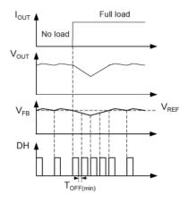
Figure 3. MIC26950 Load Transient Response
