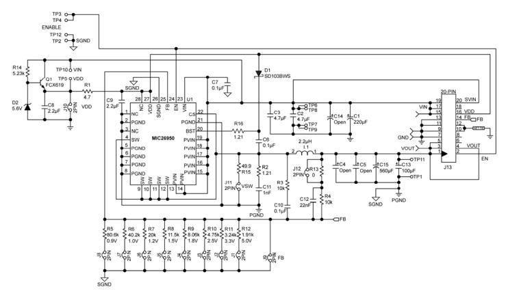
Figure 8. Schematic of MIC26950 Evaluation Board (J13, R13, R15 are for testing purposes)
