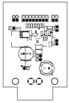
Figure 10. MIC26950 Evaluation Board Mid-Layer 1 (Ground Plane)
