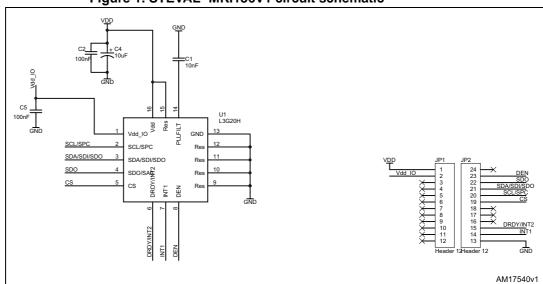
Figure 1. STEVAL- MKI136V1 circuit schematic
