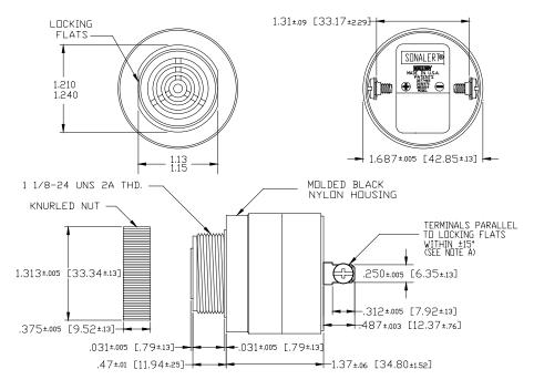
NOTE A: TERMINALS-.032 BRASS TIN PLATED, TAPPED FOR #6-32 SCREW. TWO #6-32 NICKEL PLATED BRASS SCREWS INCLUDED. WILL ACCEPT 1/4" QUICK CONNECT. NOTE B: MOUNTING- REMOVE BLACK PLASTIC NUT AND INSERT THREADED FRONT THROUGH 1.25" HOLE PUNCHED IN PANEL, IF ORIENTATION IS NEEDED, NOTE LOCKING FLATS ON DRAWING. SCREW NUT BACK ON. DO NOT OVERTIGHTEN.
