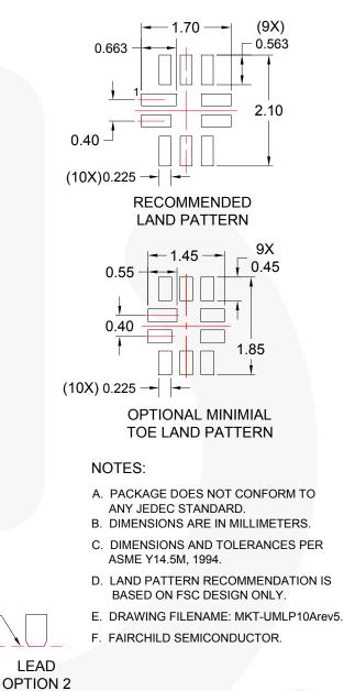
Figure 19. 10-Lead, Ultrathin Molded Leadless Package (UMLP)
