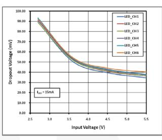
Figure 9. Dropout Voltage vs. Input Voltage
