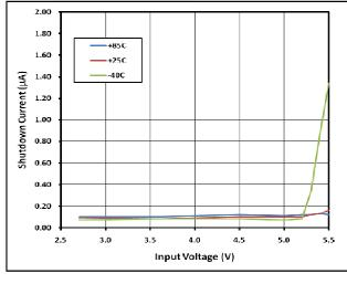
Figure 12. Shutdown Current vs. Input Voltage
