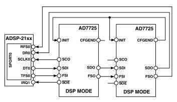
Figure 33. Daisy-Chaining Devices with a Common DSP
