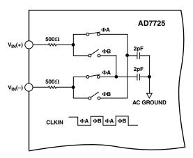
Figure 11. Analog Input Equivalent Circuit
