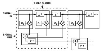
b) FIR Postprocessor Implementation Figure 20. AD7725 Postprocessor Mapping
