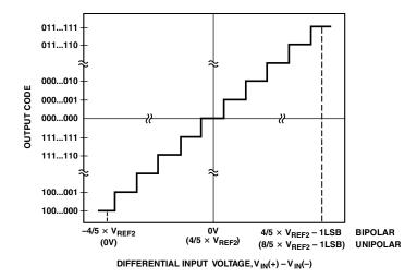
Figure 10. Bipolar/(Unipolar) Mode Transfer Function
