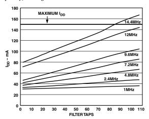
Figure 24. Typical  $I_{DD}$  vs. Filter Taps for Various CLKIN Frequencies
