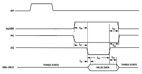
Figure 7. Parallel Mode (Reading Data from the AD7725)
