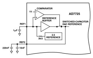
Figure 15. Reference Circuit Block Diagram
