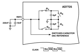
Figure 16. REF2 Equivalent Input Circuit
