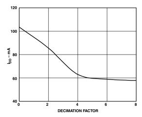
Figure 22. I<sub>DD</sub> vs. Decimation for a Filter with a Transition Width of 66 kHz as Shown in Figure 1
