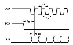
Figure 5. Serial Mode (EPROM Mode)
