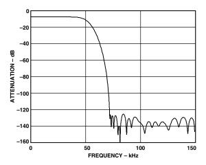
Figure 21. Default Filter Response for CLKIN = 9.6 MHz
