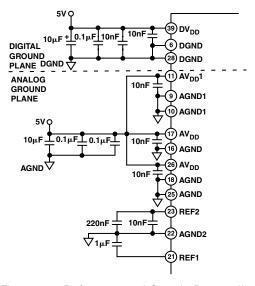
Figure 36. Reference and Supply Decoupling
