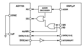
Figure 25. AD7725 Parallel Interface to Microprocessor
