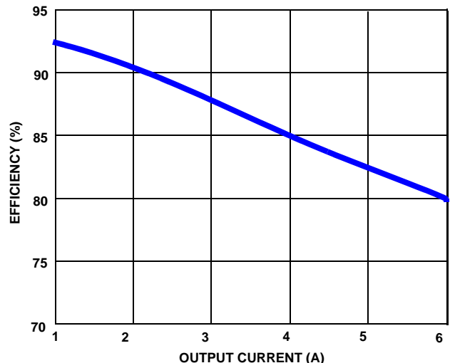
FIGURE 8. EFFICIENCY vs LOAD CURRENT
