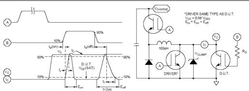
Figure 15, Switching Loss Test Circuit and Waveforms
