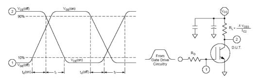
Figure 16, Resistive Switching Time Test Circuit and Waveforms
