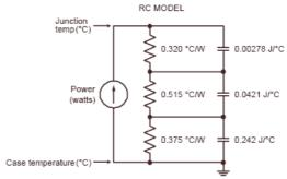
FIGURE 1b, TRANSIENT THERMAL IMPEDANCE MODEL
