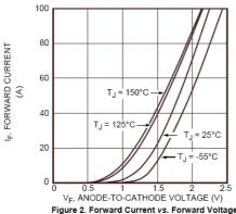
Figure 2. Forward Current vs. Forward Voltage
