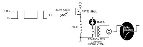
Figure 9. Diode Test Circuit
