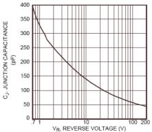
Figure 8. Junction Capacitance vs. Reverse Voltage
