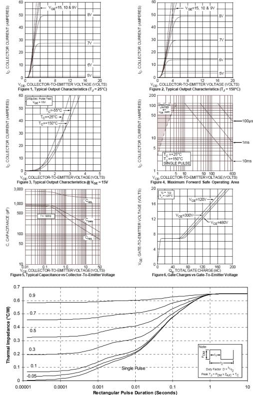
Figure 7, Maximum Effective Transient Thermal Impedance, Junction to Case vs Pulse Duration
