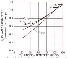
Figure 6. Dynamic Parameters vs. Junction Temperature
