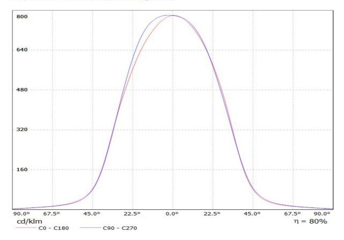
Luminaire: LEDiL Oy CN13115\_LENINA-W-DL\_(SoleriqE30) Eff.80.2% Lamps: 1 x Osram Soleriq E30 (1262.22Im@250mA)
