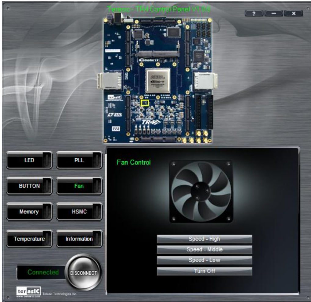
Figure 3-12 Fan Control of the TR4
