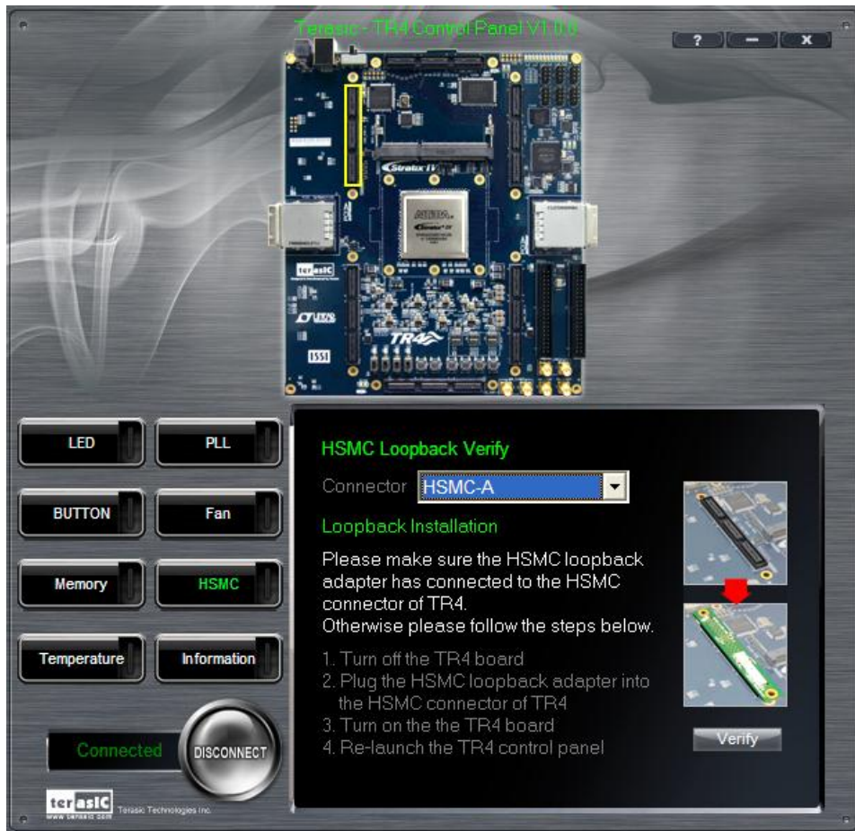
Figure 3-11 HSMC Loopback Verification Test Performed under Control Panel
