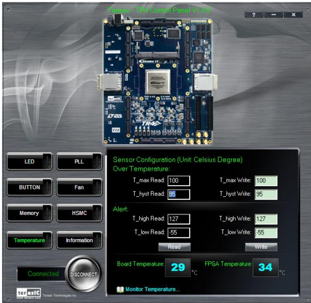
Figure 3-9 Accessing the Temperature Sensor through Control Panel
