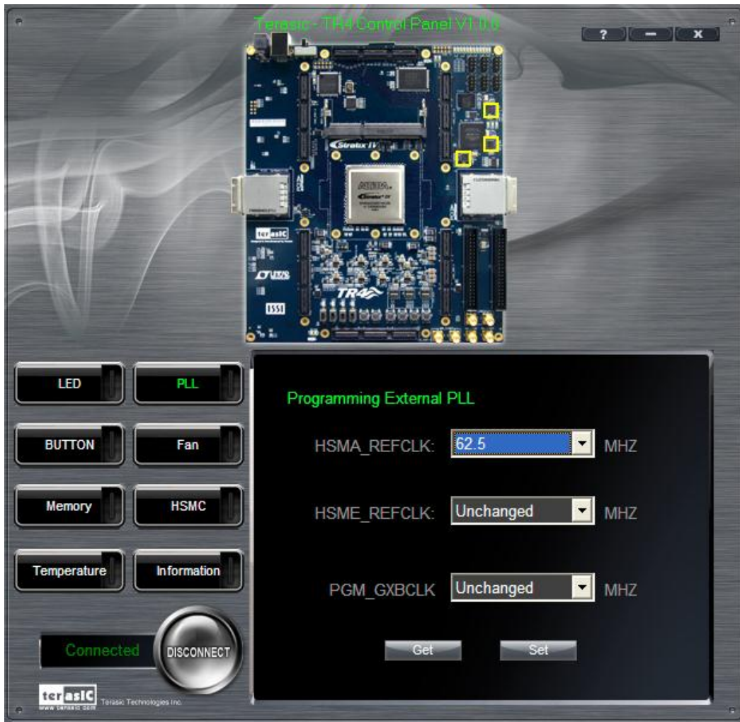
Figure 3-10 Programmable External PLL Configured through Control Panel
