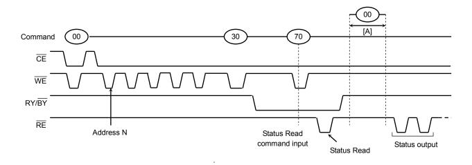
The device status can be read out by inputting the Status Read command "70h" in Read mode. Once the device has been set to Status Read mode by a "70h" command, the device will not return to Read mode unless the Read command "00h" is inputted during [A]. If the Read command "00h" is inputted during [A], Status Read mode is reset, and the device returns to Read mode. In this case, data output starts automatically from address N and address input is unnecessary
