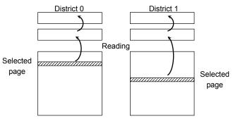
The data transfer operation from the cell array to the Data Cache via Page Buffer starts on the rising edge of  $\overline{WE}$  in the 30h command input cycle (after the 2 Districts address information has been latched). The device will be in the Busy state during this transfer period.
