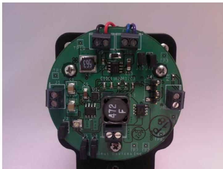
Figure 5: Completed electrical connections on DK-105T-1
