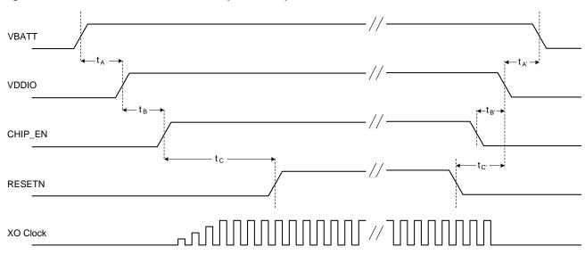
Figure 5-1. ATWINC3400-MR210 Power-up/down Sequence
