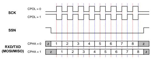
Figure 10-2. ATWINC3400-MR210 SPI Slave Clock Polarity and Clock Phase Timing
