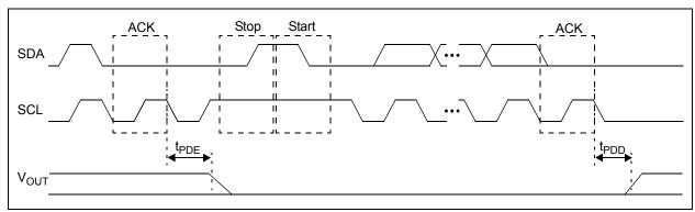
**FIGURE 1-3:**  $l^2C^{TM}$  Power-Down Command Timing.
