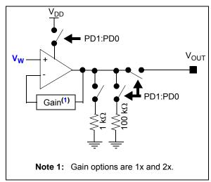
FIGURE 5-5: Output Driver Block Diagram.
