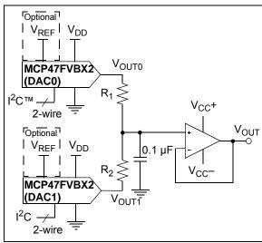
FIGURE 8-7: Simple Double Precision DAC using MCP47FVBX2.
