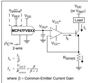
FIGURE 8-8: Digitally-Controlled Current Source.
