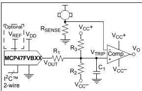
FIGURE 8-4: Single-Supply "Window" DAC.
