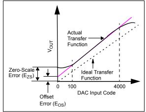
**FIGURE C-2:** Offset Error (Zero Gain Error).
