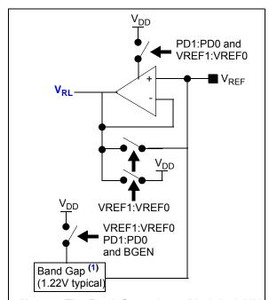
Note 1: The Band Gap voltage (V<sub>BG</sub>) is 1.22V typical. The band gap output goes through the buffer with a 2x gain to create the V<sub>RL</sub> voltage. See **Section 5.4 "Internal Band Gap"** for addition information on the band gap circuit.
