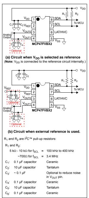
FIGURE 8-2: Example Circuit.
