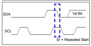
FIGURE B-5: Repeat Start Condition Waveform.
