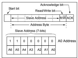
**FIGURE 6-2:** Slave Address Bits in the  $l^2$ C Control Byte.
