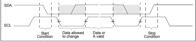
**FIGURE B-8:**  $l^2C$  Data States and Bit Sequence.
