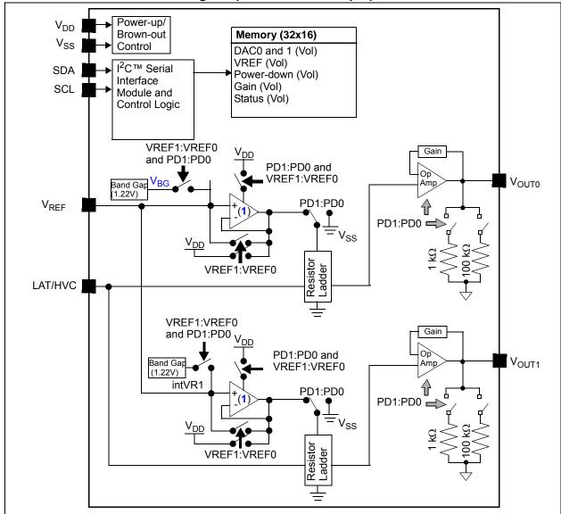
Note 1: If Internal Band Gap is selected, this buffer has a 2x gain. If the G bit = '1', this is a total gain of 4.
