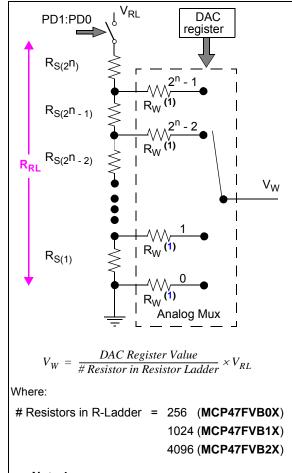
**Note 1:** The analog switch resistance (R<sub>W</sub>) does not affect performance due to the voltage divider configuration.
