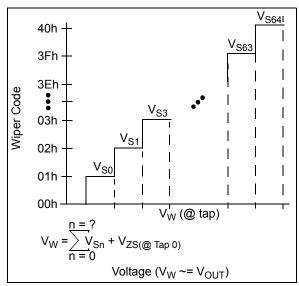
FIGURE C-1:  $V_W(V_{OUT})$
