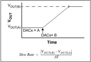
FIGURE 5-6: V<sub>OUT</sub> Pin Slew Rate.
