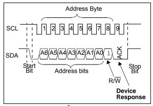
**FIGURE 8-1:** I<sup>2</sup>C Bus Connection Test.
