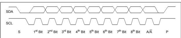
FIGURE B-7: Typical 8-Bit I<sup>2</sup>C Waveform Format.
