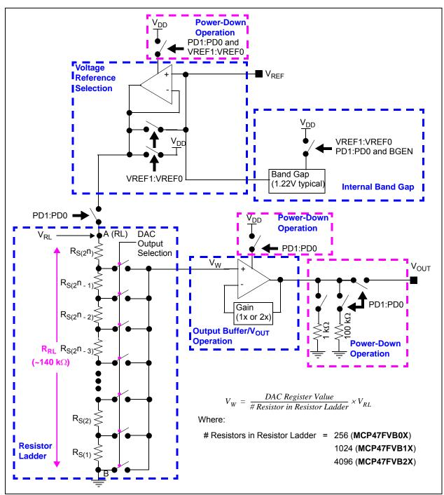
FIGURE 5-1: MCP47FVBXX DAC Module Block Diagram.
