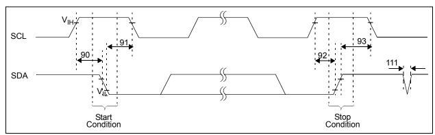
**FIGURE 1-5:**  $l^2C^T$  Bus Start/Stop Bits Timing Waveforms.
