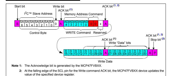
3: This command sequence does not need to terminate (using the Stop bit), and the Write command can be repeated (see continuous write format, Section 7.1.2 "Continuous Writes to Volatile Memory").
