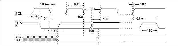
**FIGURE 1-6:**  $I^2C^{TM}$  Bus Timing Waveforms.
