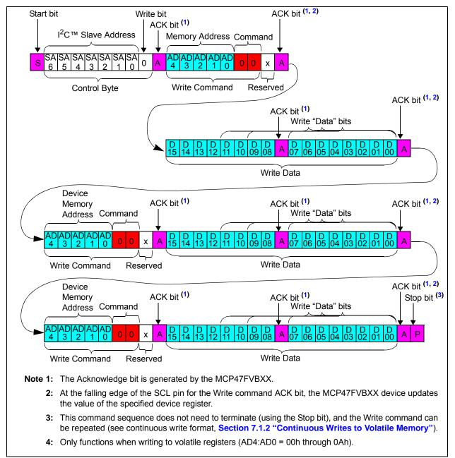
FIGURE 7-3: Continuous Write Commands.
