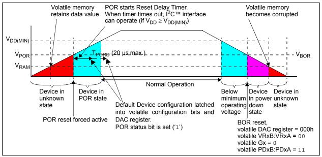
FIGURE 4-1: Power-on Reset Operation.
