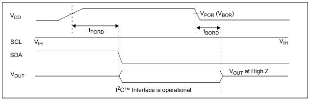
FIGURE 1-2: Power-on and Brown-out Reset Waveforms.
