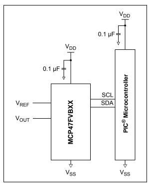
**FIGURE 8-10:** Typical Microcontroller Connections.
