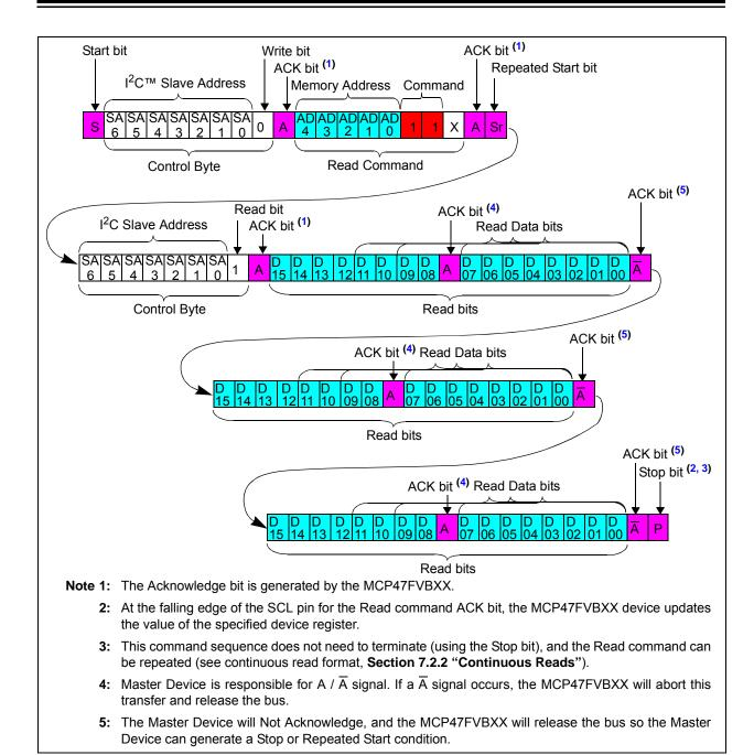
FIGURE 7-7: Continuous Read Command Of Specified Address.
