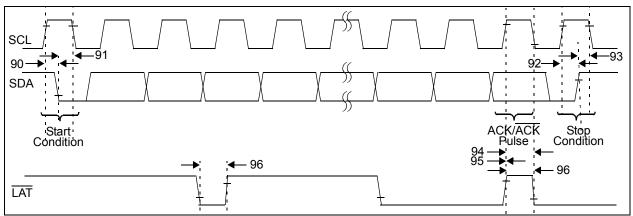
**FIGURE 1-4:**  $l^2C^{TM}$  Bus Start/Stop Bits Timing Waveforms.
