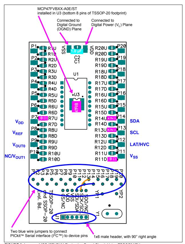
FIGURE 9-1: MCP47FVBXX Evaluation Board Circuit Using TSSOP20EV.
