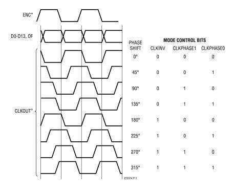
Figure 11. Phase Shifting CLKOUT
