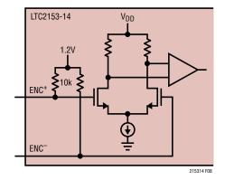
Figure 8. Equivalent Encode Input Circuit
