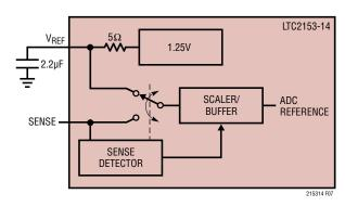
Figure 7. Reference Circuit
