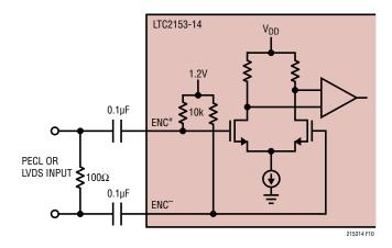
Figure 10. PECL or LVDS Encode Drive
