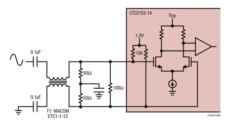
Figure 9. Sinusoidal Encode Drive
