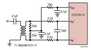
Figure 3. Analog Input Circuit Using a Transformer.
