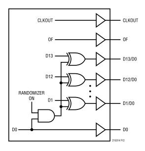
Figure 12. Functional Equivalent of Digital Output Randomizer
