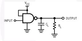
$C_L$  includes load and stray capacitance Input PRR = 1.0MHz,  $t_{\rm W}$  = 500ns
