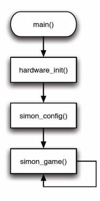
After all configuration is complete, we move into the core simon\_game() routine. Immediately after entering simon\_game(), the system is configured to enter a low-power sleep mode and to awake on a button press from any of the four buttons. Sleep mode is attained by calling a specific sequence of functions/macros, which define the type of sleep mode we want to enter, configuring the interrupts, and then going to sleep:
