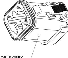
PLUG, 6 SOCKET, AT SERIES, SOLID REAR SEAL, END CAP
