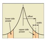
Additionally, the user can select from any of the following three measurement methods, based on the carrier wave definition: Total power, Peak (reference level) and in-band.
