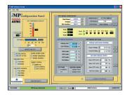
Setting-up an iMP power module could not be simpler. The same control screen is used for all modules and all operating parameters. So as well as defining a module's output voltage and current, you can just as easily adjust its OVP, UVP and OTP limits, change its OCP mode and control signal, and force fan speed override if required. All with clear on-screen confirmation and feedback.
