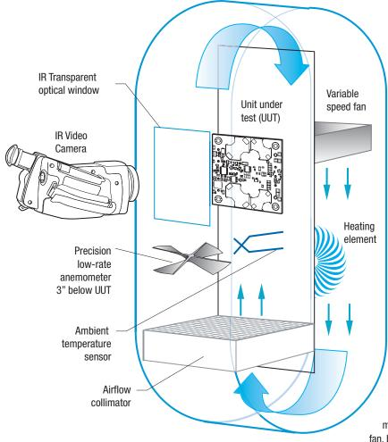
Figure 12. Vertical Wind Tunnel
