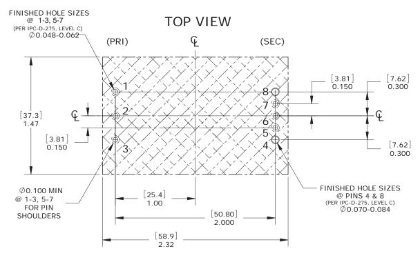
IT IS RECOMMENDED THAT NO PARTS BE PLACED BENEATH CONVERTER (HATCHED AREA)
