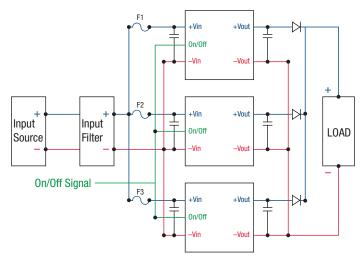
Figure 4. Redundant Parallel Connections
