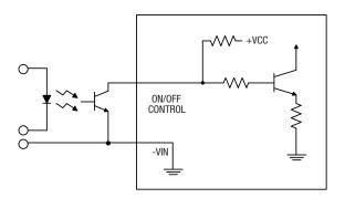
Figure 7. Driving the On/Off Control Pin (suggested circuit)
