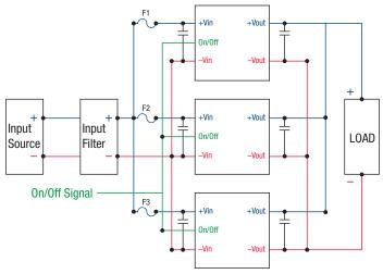
Figure 2. Load Sharing Block Diagram
