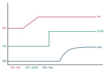
Figure 3. Typical Turn On for Positive Logic Modules
