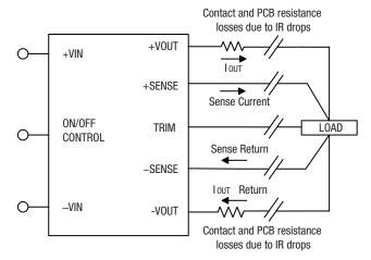
Figure 11. Remote Sense Circuit Configuration
