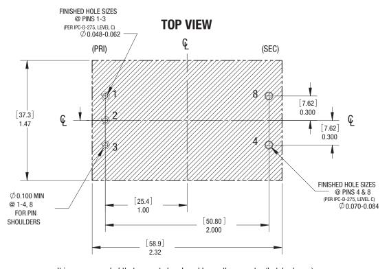
It is recommended that no parts be placed beneath converter (hatched area).
