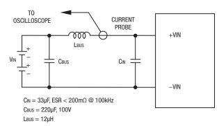
Figure 5. Measuring Input Ripple Current
