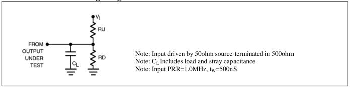
Figure 1. AC Test Circuit
