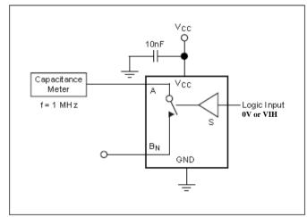
Figure 8. Channel On Capacitance
