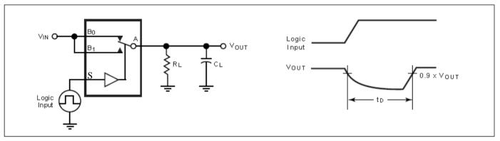
Figure 3. Break Before Make Interval Timing
