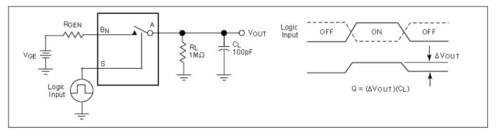
Figure 4. Charge Injection Test
