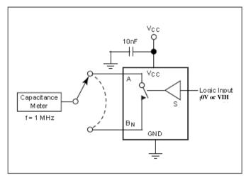
Figure 7. Channel Off Capacitance
