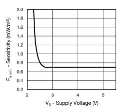
Fig. 9 - Sensitivity vs. Supply Voltage
