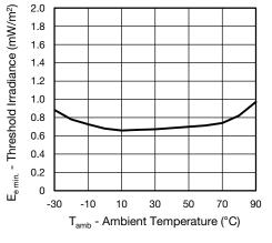
Fig. 6 - Sensitivity vs. Ambient Temperature
