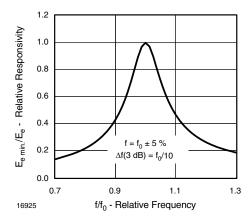
Fig. 5 - Frequency Dependence of Responsivity
