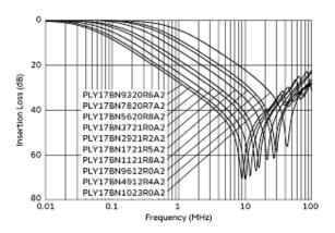
Common Mode Insertion Loss-Frequency Characteristics
