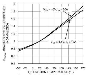
Figure 6. On-Resistance Variation with Temperature
