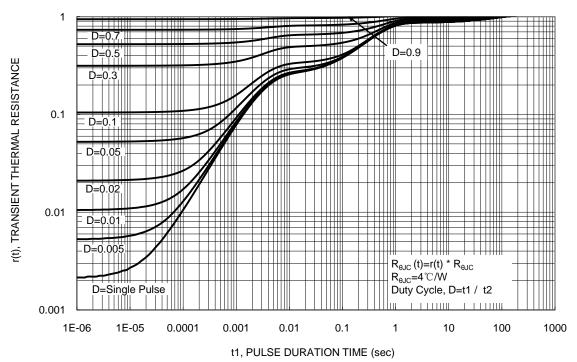
Figure 13. Transient Thermal Resistance
