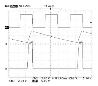
Figure 6. The Fault Condition Is Triggered when the UV Pin Voltage Falls Below 1.0 V. The Soft-Start Capacitor Is Discharged and the GATE Output Is Disabled. CH2: Envelop of GATE Output, CH3: SS Pin with 0.01 µF Capacitor, CH4: UV Pin
