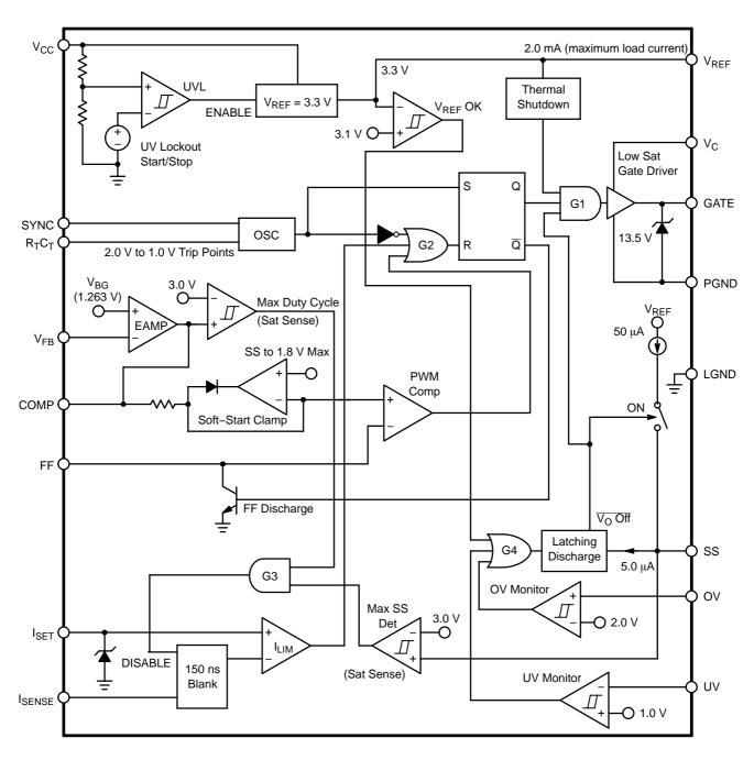
Figure 2. Block Diagram
