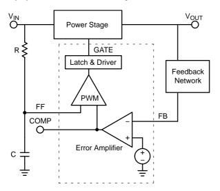
Figure 3. Feed Forward Voltage Mode Control
