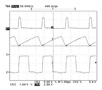
Figure 8. The SYNC Pin Generates a Sync Pulse at the Beginning of Each Switching Cycle. CH2: GATE Pin, CH3: R<sub>T</sub>C<sub>T</sub>, CH4: SYNC Pin
