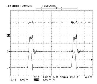
Figure 7. The GATE Output Is Terminated When the I<sub>SENSE</sub> Pin Voltage Reaches the Threshold Set By the I<sub>SET</sub> Pin. CH2: I<sub>SENSE</sub> Pin, CH4: I<sub>SET</sub> Pin, CH3: GATE Pin
