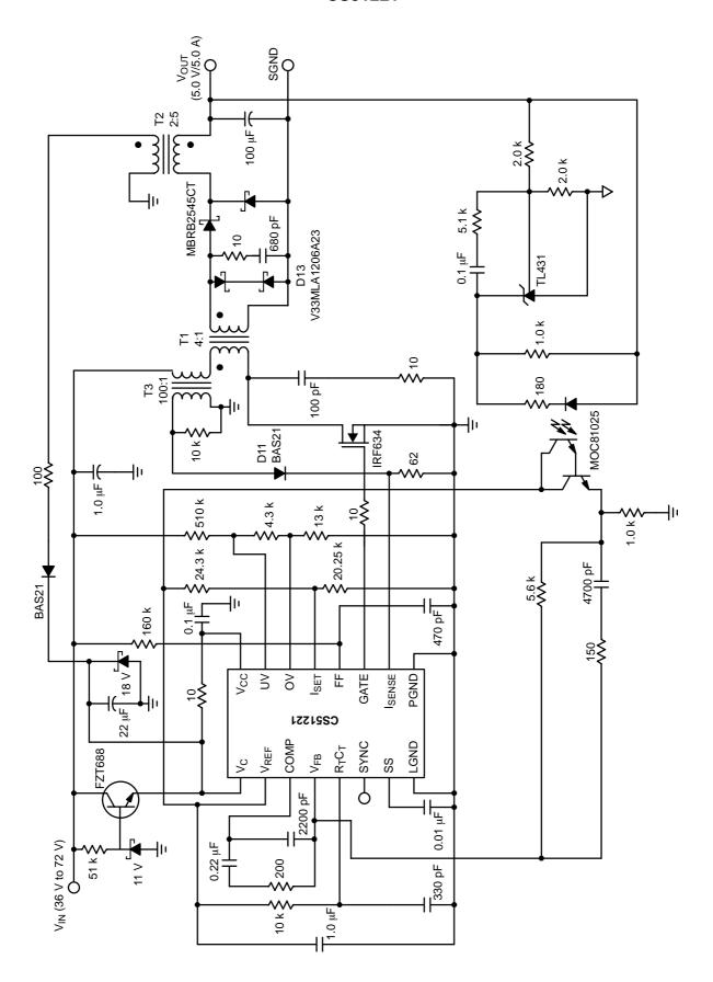
Figure 1. Application Diagram, 36 V-72 V to 5.0 V/5.0 A Converter
