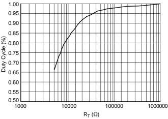
Figure 11. Typical Performance Characteristics, Oscillator Duty Cycle vs. R<sub>T</sub>
