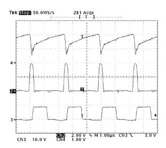
Figure 9. Operation with External Sync. CH2: SYNC Pin, CH3: GATE Pin, CH4: R<sub>T</sub>C<sub>T</sub> Pin
