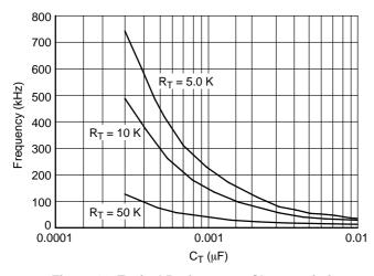
Figure 10. Typical Performance Characteristics, Oscillator Frequency vs. C<sub>T</sub>
