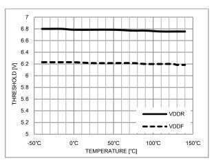
Figure 12. V<sub>DD</sub> UVLO Threshold vs. Temperature
