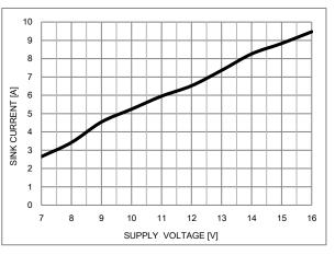
Figure 22. HO, LO Peak Sink Current vs. Supply Voltage
