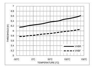
Figure 13. VHB UVLO Threshold vs. Temperature
