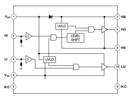
Figure 3. Simplified Block Diagram
