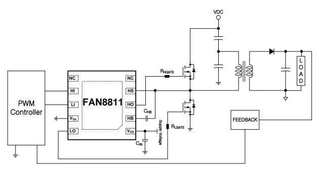
Figure 2. Application Schematic – Half Bridge Converter
