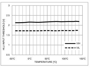
Figure 10. Input Threshold vs. Temperature
