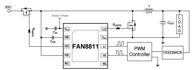
Figure 1. Application Schematic – Synchronous Buck Converter
