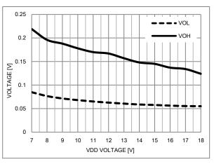
Figure 16.  $V_{OH}$ ,  $V_{OL}$  Voltage vs.  $V_{DD}(V_{HB})$
