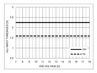
Figure 11. Input Threshold vs. V<sub>DD</sub>
