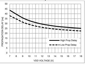
Figure 20. High Side Propagation Delay vs. VHB
