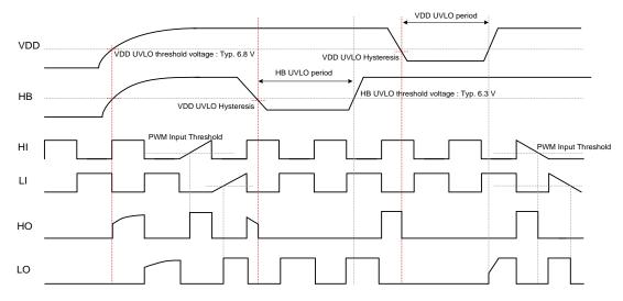
Figure 24. Overall Operation Timing Diagram
