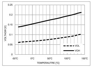
Figure 15. V<sub>OH</sub>, V<sub>OL</sub> Voltage vs. Temperature
