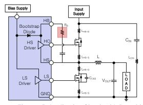
Figure 25. Application Circuit with Parasitic Components
