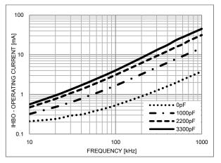
Figure 9. IHB Operating Current vs. Frequency
