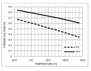
Figure 14. Bootstrap Diode VF vs. Temperature
