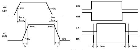
Figure 23. Timing Diagrams
