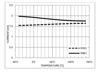
Figure 7. Operating Current vs. Temperature
