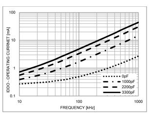
Figure 8. IDD Operating Current vs. Frequency
