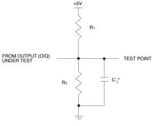
$^{\star}\mathrm{C}_{\,\mathrm{L}}$  INCLUDES TEST FIXTURE AND PROBE CAPACITANCE
