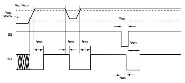
FIGURE 2. POWER SUPPLY MONITORING DIAGRAM
