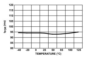
FIGURE 6. tpor vs TEMPERATURE
