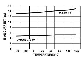
FIGURE 7. BIAS CURRENT vs TEMPERATURE
