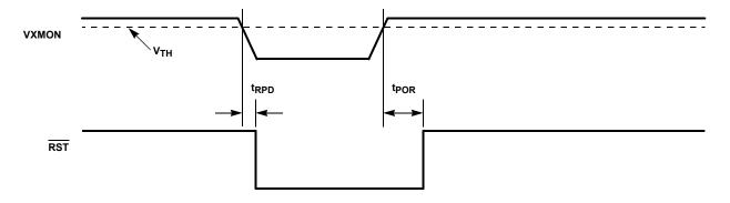
FIGURE 3. VOLTAGE MONITORING DIAGRAM
