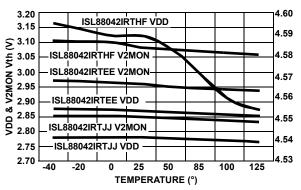
FIGURE 4. VDD and V2MON Vth vs TEMPERATURE
