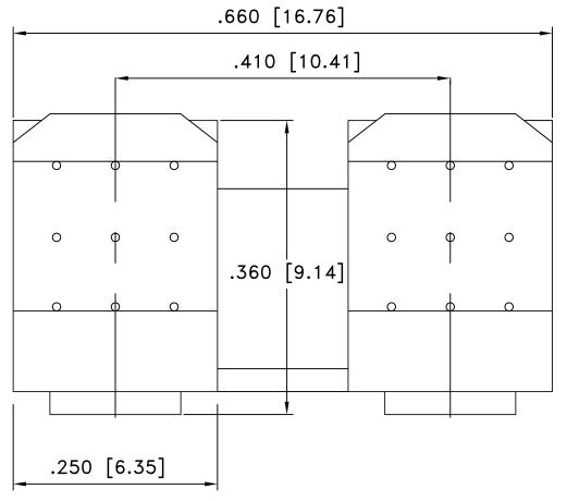
MATERIAL: 0.010" SPRING TEMPER STAINLESS STEEL, NICKEL PLATED ROHS COMPLIANT
