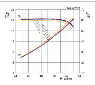
$V_{DS}$  = 28 V;  $I_{Dq}$  = 1200 mA;  $t_p$  = 10  $\mu$ s;  $\delta$  = 10 %.
