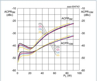
$V_{DS}$  = 28 V;  $I_{Dq}$  = 1200 mA.
