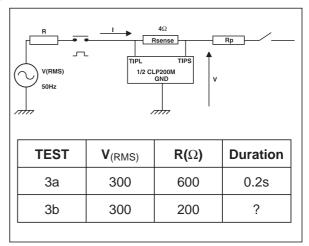
**Fig. 17 :** CLP200M response to the induction test (Test 3a).
