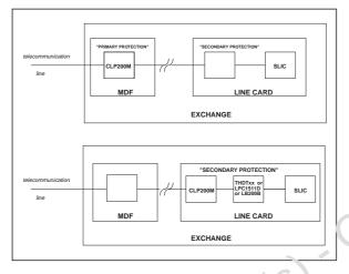
Figure 1 is a simplified block diagram of a subscriber line protection that is mainly used so far.
