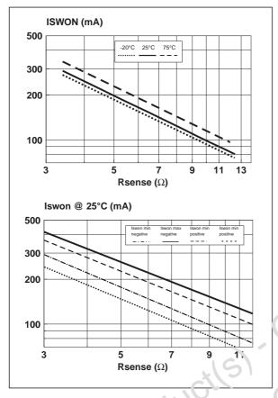
The choice of the switching-cr. current is function of the  $R_{SENSE}$  resistors.
