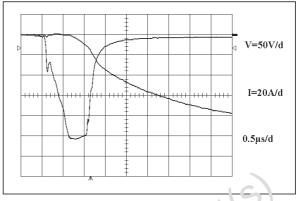
Figures 14 and 15 show that the remaining overvoltage does not exceed -260 V. The CLP200M switches on with:  $0.7 \ \mu$ s and withstands the 100 A given by the CCITT K20 generator.
