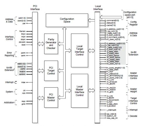
Note: Signals in shaded boxes are used for 64-bit PCI Cores.
