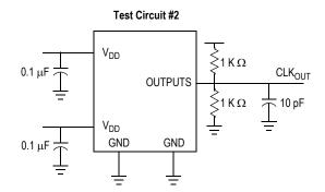
Test Circuit for t<sub>8</sub>, Output slew rate on -1H, -5 device
