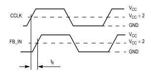
Figure 2. Static Phase Offset Test Reference
