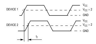
Figure 4. Device-to-Device Skew
