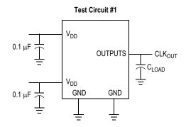
Test Circuit for all parameters except t<sub>8</sub>
