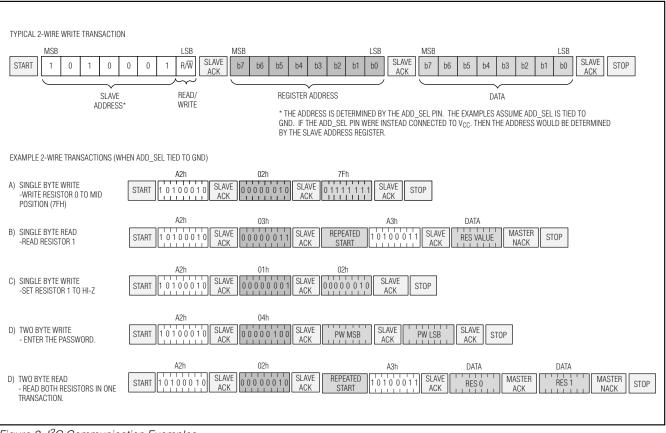
Figure 2. I<sup>2</sup>C Communication Examples
