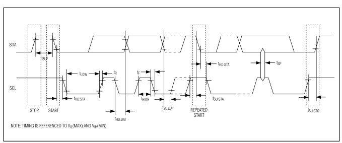
Figure 1. I<sup>2</sup>C Timing Diagram
