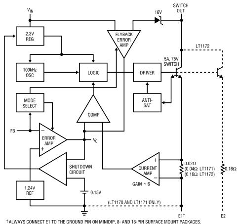
ALWAYS CONNECT E1 TO THE GROUND PIN ON MINIDIP, 8- AND 16-PIN SURFACE MOUNT PACKAG E1 AND E2 INTERNALLY TIED TO GROUND ON TO-3 AND TO-220 PACKAGES.
