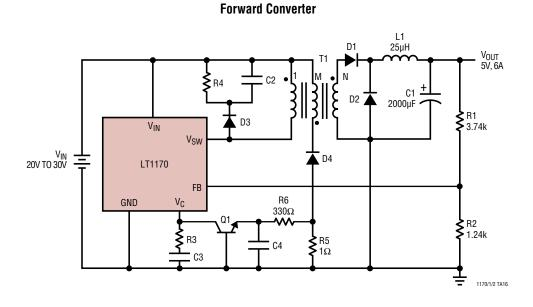
**High Efficiency 5V Buck Converter**
