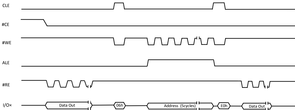
Figure 9-4 Two Plane Random Data Read (06h-E0h) Operation
